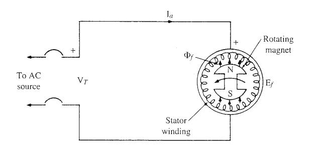
Rotating field flux Φ<sub>f</sub> due to magnetic field in the rotor. A "speed" voltage, "counter-emf", or "excitation" voltage E<sub>f</sub> is generated and acts in opposition to the applied voltage.
