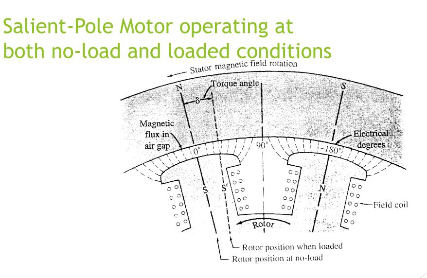
Angle  $\delta$  is the *power angle*, *load angle*, or *torque angle*
